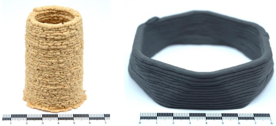
Fig. 5. Printed parts from wood paste (l) and geopolymer (r)
